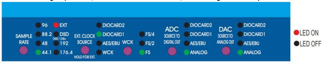
In this mode both the AD and DA run on an external clock. Although this mode does not provides the lowest jitter performance it might be desirable for systemic reasons. For example a second 8X192 unit running can be coupled with a master 8X192 unit via a Firewire cable only. In this case the clock for second unit is provided via Firewire card (DIOCARD1 in this example).
