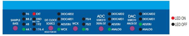
In this mode both the AD and DA run on an external clock. Holding the "Ext. Clock Source" button selects this mode. Although this mode does not provide the lowest jitter performance it might be desirable for systemic reasons. External recorders (such as DAW etc) can be synchronized to external wordclock sources OR AD digital outputs (any format: AES or DIOCARD1 or DIOCARD2) OR to converter Worclock output.
