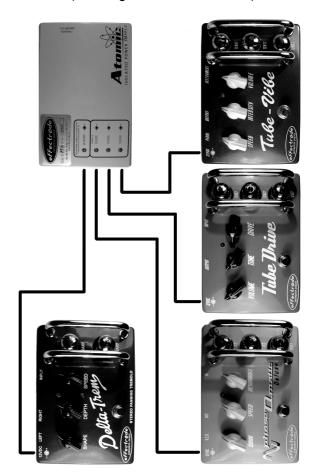
The first power output can be used to power 9V center negative pedals in a daisy-chain as shown below.
