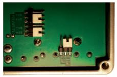
To configure for 9V center negative pedals set the jumpers as shown below.
