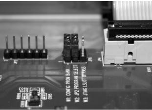
If you are updating a Rev B Aurora, slide switch 4 (labeled W4 on PCB) of SW1 to the OFF position (towards back panel)
