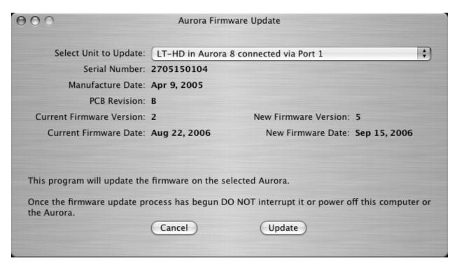
When the update process is complete, it is important to press the Power button to shut down the Aurora AND then **disconnect the Aurora from its power source**.
