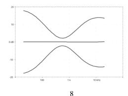
**BRIGHT** – The bright is an advanced high pass filter capable of producing bright high treble timbre, without adding practically any noise. It gives 12dB boost at 10kHz and may give brightness to old passive pickups.
