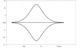
**EDGE FILTER** – The EDGE filter is a 'bell' type filter peaking at around 7kHz controlling the higher mids and treble registers, giving presence and "edge".
