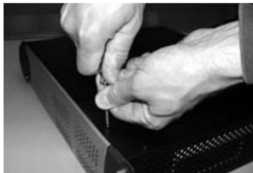
Removing the top cover screws
