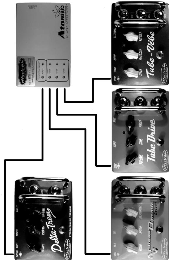
The first power output can be used to power 9V center negative pedals in a daisy-chain as shown below.
