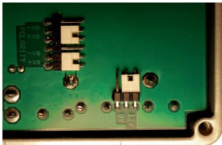
To configure for 9V center negative pedals set the jumpers as shown below.
