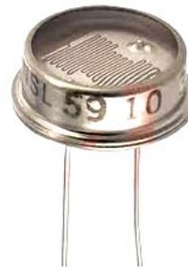
The release time of the compressor is entirely determined by the photocell in the attenuator. The cell has a desirable two-stage decay characteristic where it releases within 40 to 80ms to approximately half its off resistance when light is absent. The remainder of the release
